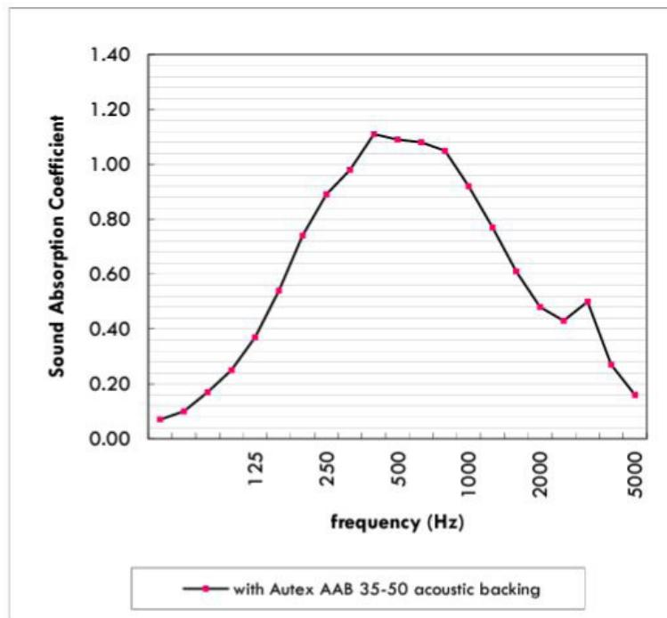
Sound absorption coefficients according to ISO354. Based on 12mm panel thickness.
