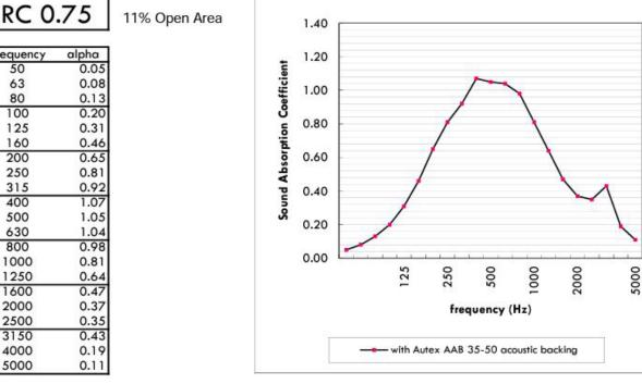
Sound absorption coefficients according to ISO354. Based on 12mm panel thickness. Margin of error is generally within +/- 0.05
