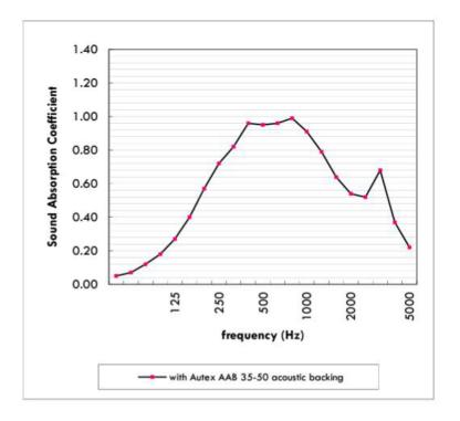
Sound absorption coefficients according to ISO354. Based on 12mm panel thickness. Margin of error is generally within +/- 0.05
