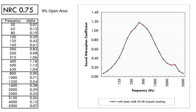
Sound absorption coefficients according to ISO354. Based on 12mm panel thickness. Margin of error is generally within +/- 0.05
