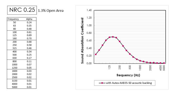
Sound absorption coefficients according to ISO354. Based on 15mm panel thickness. Margin of error is generally within +/- 0.05
