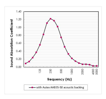
Sound absorption coefficients according to ISO354. Based on 15mm panel thickness. Margin of error is generally within  $\pm$ 0.05
