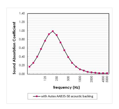
Sound absorption coefficients according to ISO354. Based on 15mm panel thickness. Margin of error is generally within  $\pm$ 0.05
