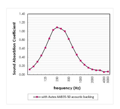
Sound absorption coefficients according to ISO354. Based on 15mm panel thickness. Margin of error is generally within +/- 0.05
