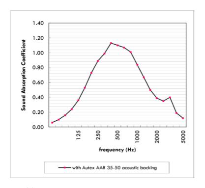
Sound absorption coefficients according to ISO354. Based on 12mm panel thickness. Margin of error is generally within  $\pm$ 0.05
