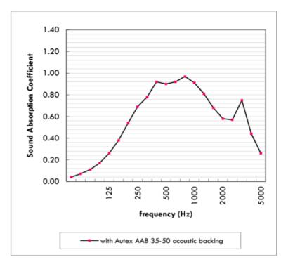
Sound absorption coefficients according to ISO354. Based on 12mm panel thickness. Margin of error is generally within +/- 0.05
