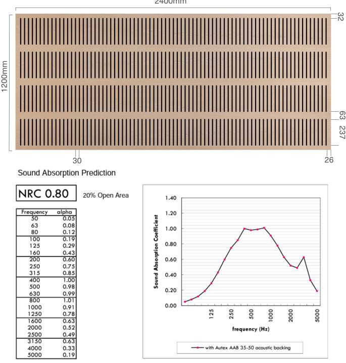
Sound absorption coefficients according to ISO354. Based on 12mm panel thickness. Margin of error is generally within +/- 0.05
