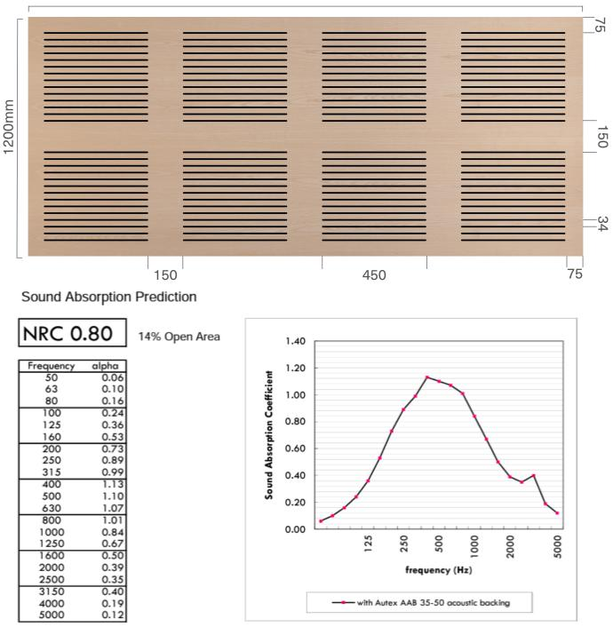
Sound absorption coefficients according to ISO354. Based on 12mm panel thickness. Margin of error is generally within +/- 0.05
